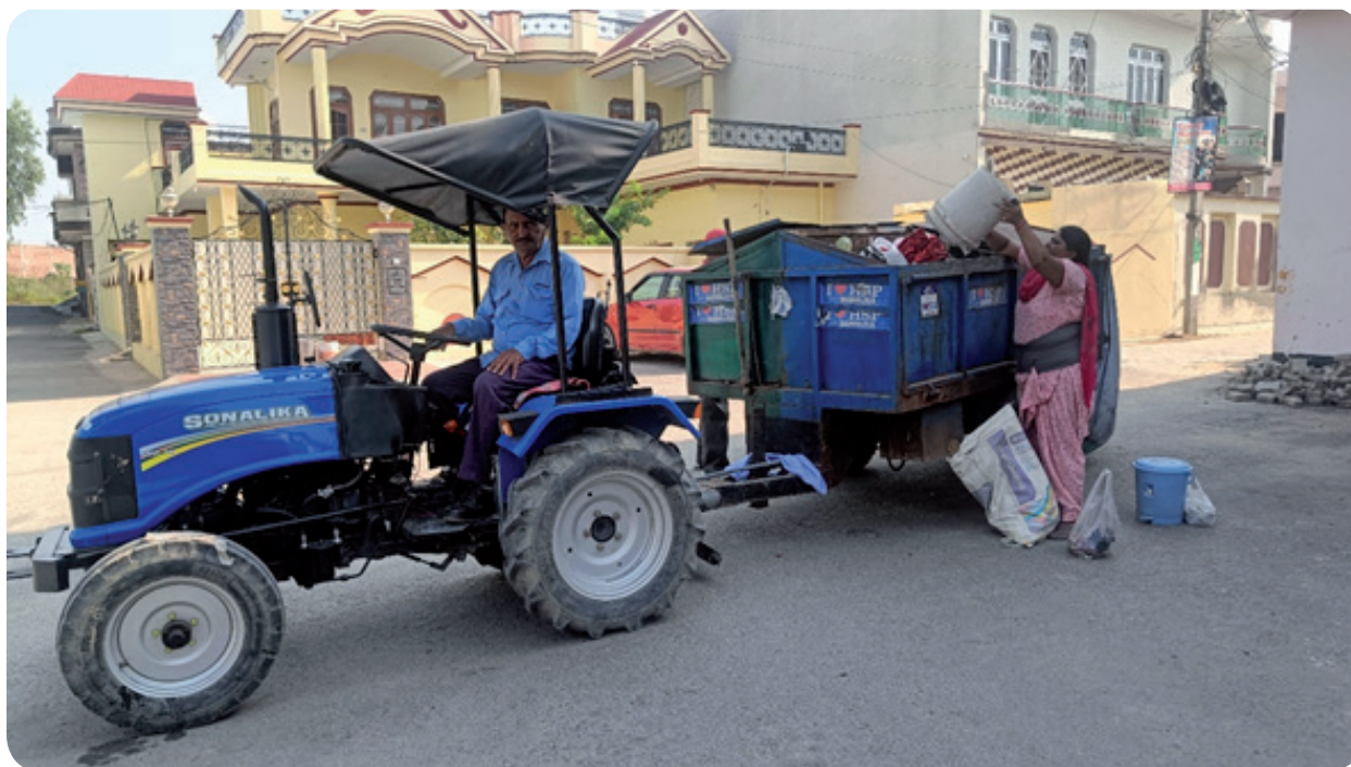
(Picture of tractor and trolley having separate compartments for dry and wet waste)
