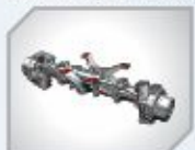
High Ground Clearance and Shorter Turning Radius with Portal Axle
