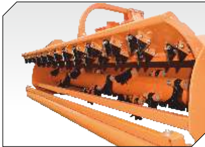
Bigger rotor drum / chamber chawing better & effective residue burning without chalking
