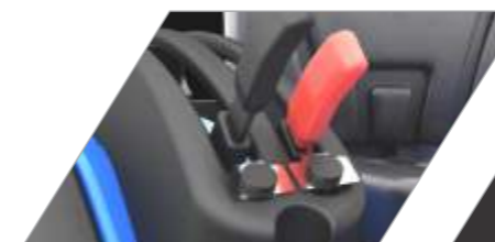
Two Lever Control - Independent Control Of Stick Draft Setting
